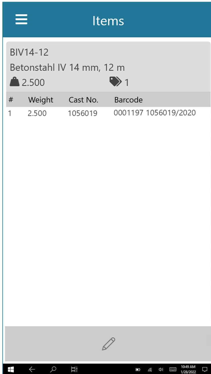
The bundles are automatically taken over with their entry weight. If this weight has to be changed, you can select the corresponding bundle and click the Edit button below.
